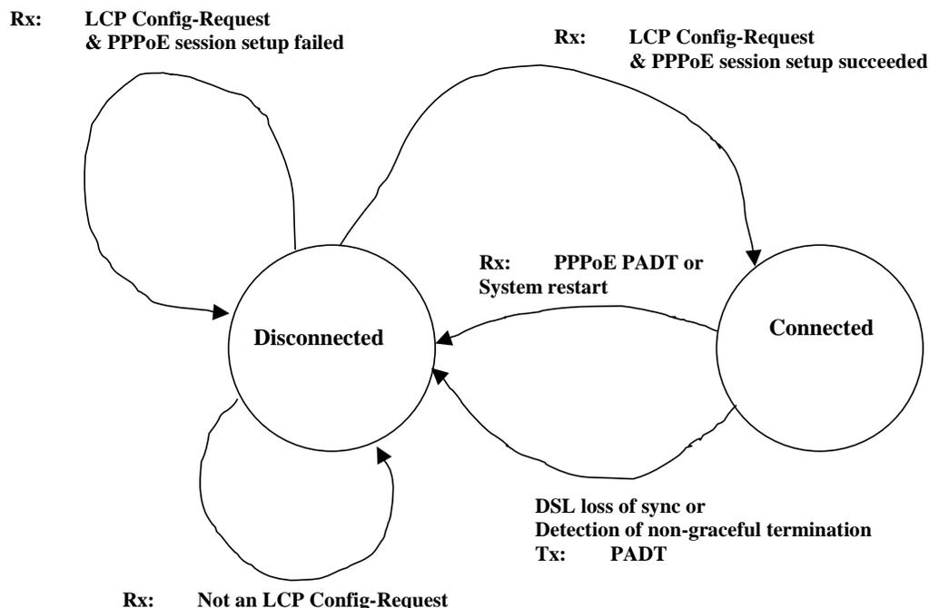
**Figure 19 - State transition diagram for PPPoA IWF**
