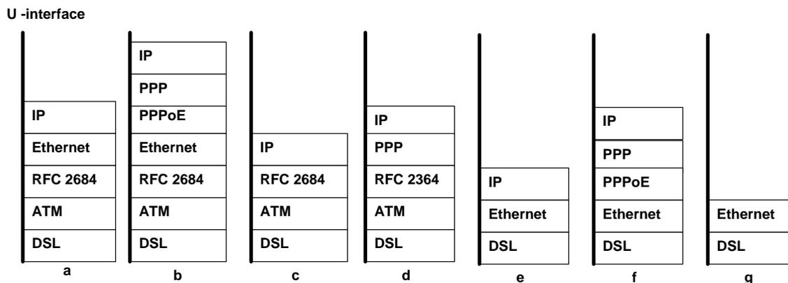
Figure 4 - Protocol stacks at the U interface
