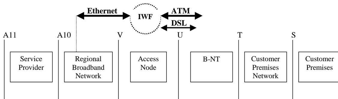
**Figure 5 - ATM to Ethernet inter-working function**
