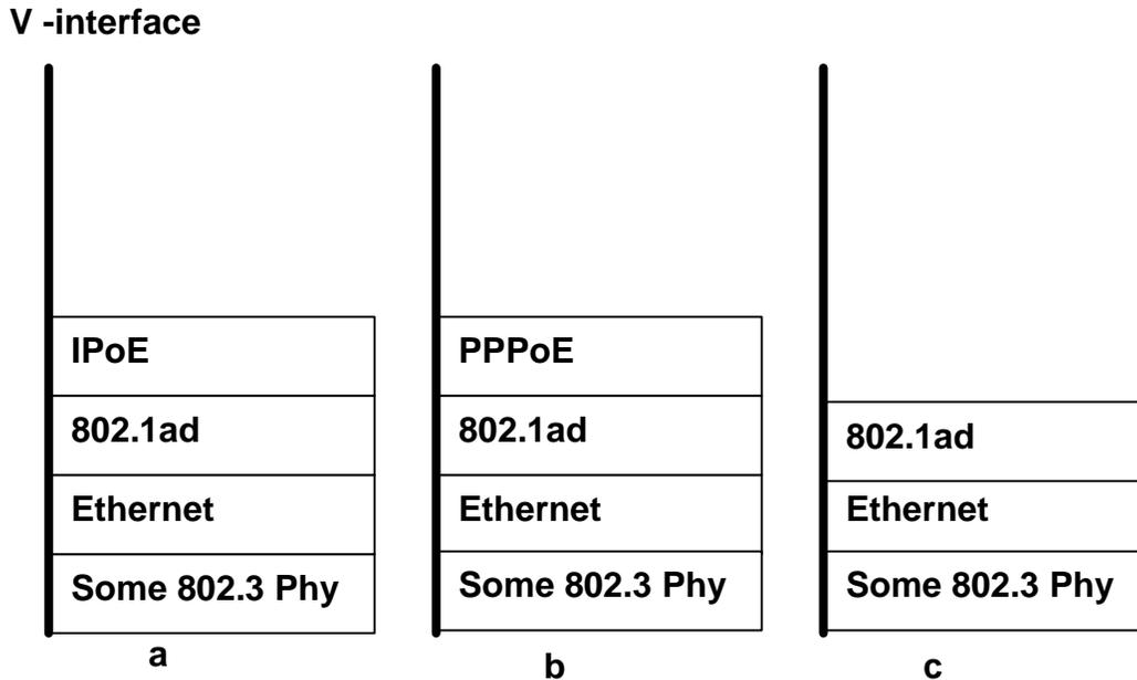
**Figure 7 - Protocol stacks at the V interface**
