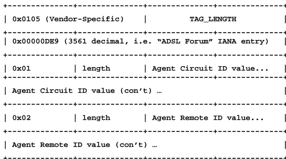
**Figure 21 - PPPoE access loop identification tag syntax**
