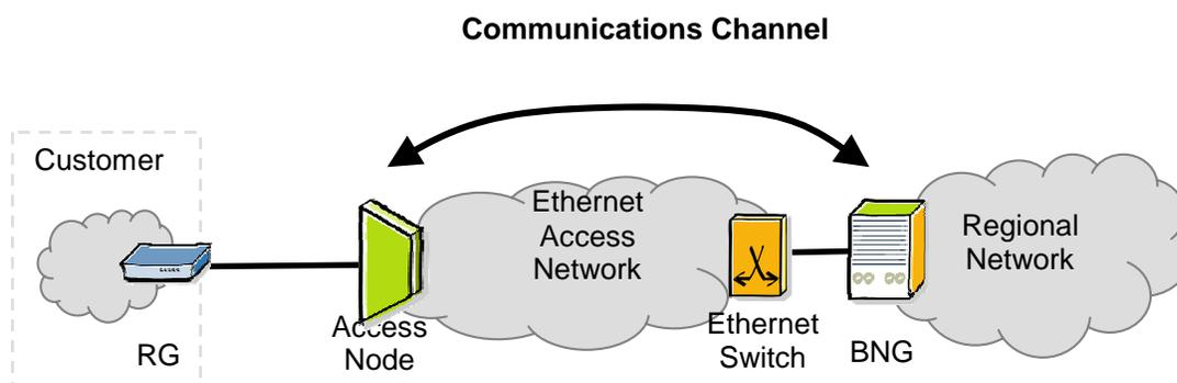
**Figure 28 - Communication channel between BNG & AN**
