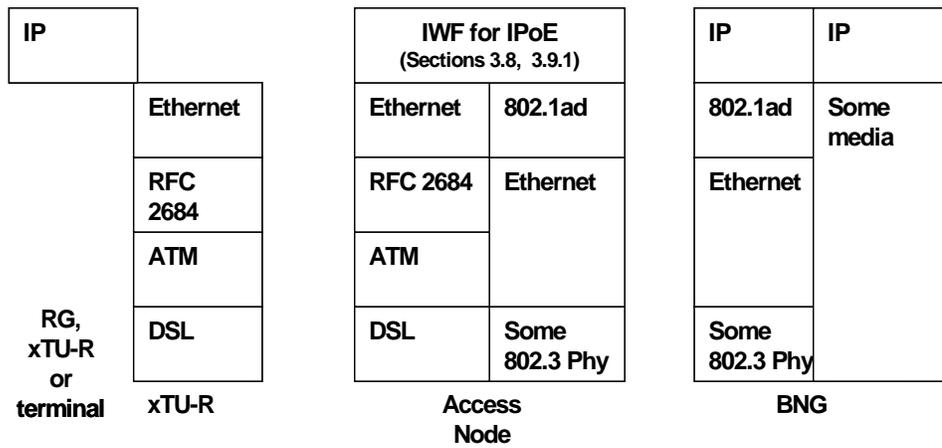
Figure 16 - End-to-end protocol processing for IPoE access
