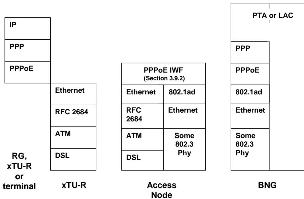
Figure 15- End-to-end protocol processing for PPPoE access
