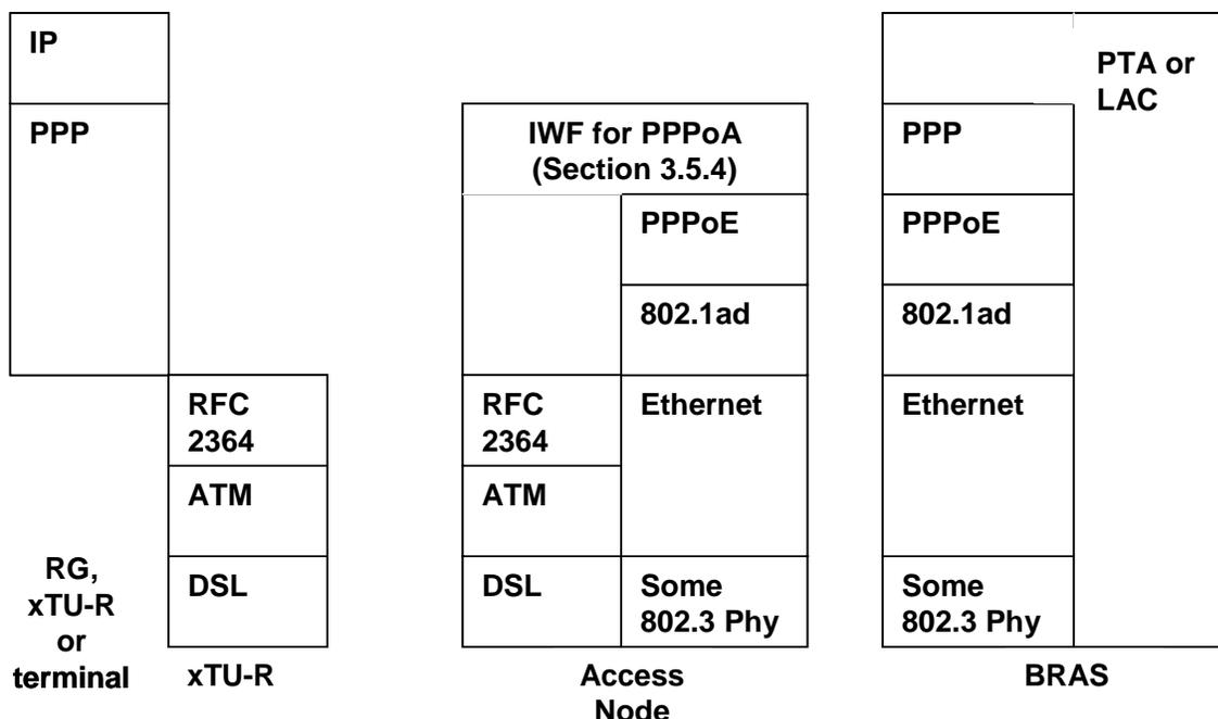
Figure 18 - End-to-end protocol processing for PPPoA access
