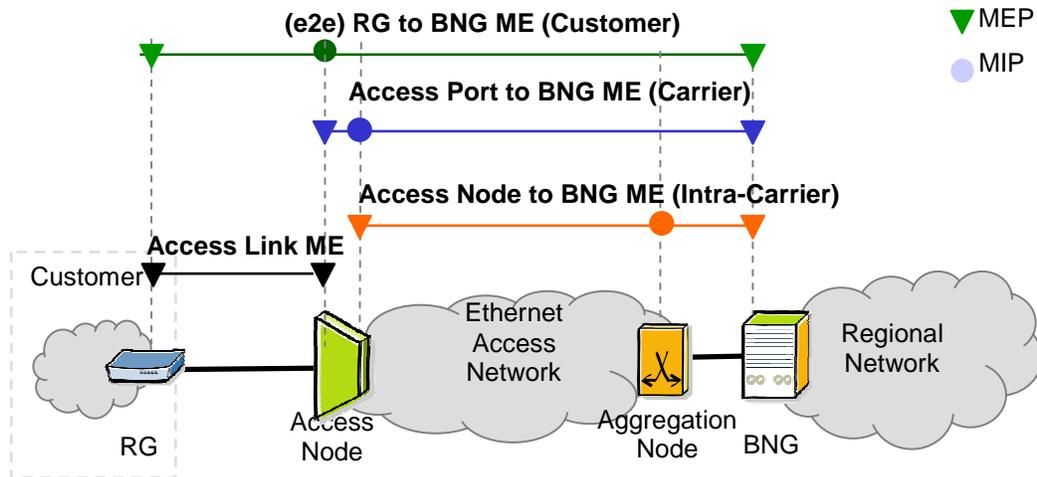
Figure 25 - Ethernet OAM model for broadband access
