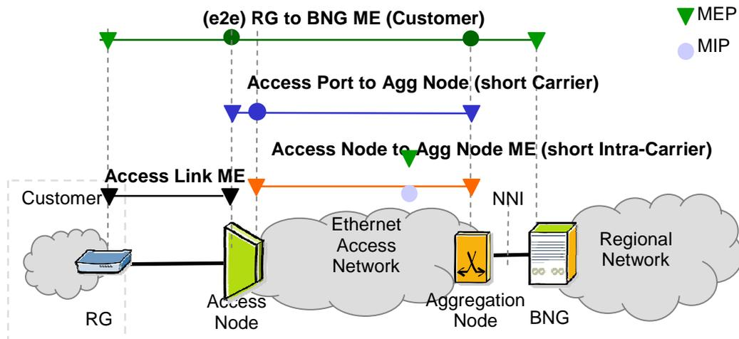
Figure 26 - Ethernet OAM model for broadband access – wholesale “Ethernet bit-stream” services model
