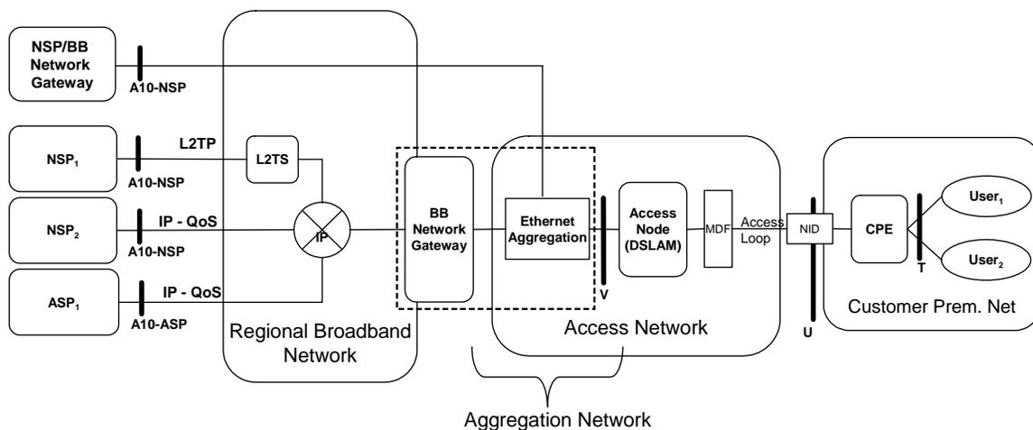
**Figure 3 – Network architecture for Ethernet-based DSL aggregation**
