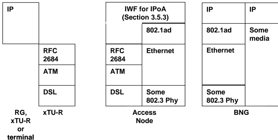
Figure 17- End-to-end protocol processing for IPoA access
