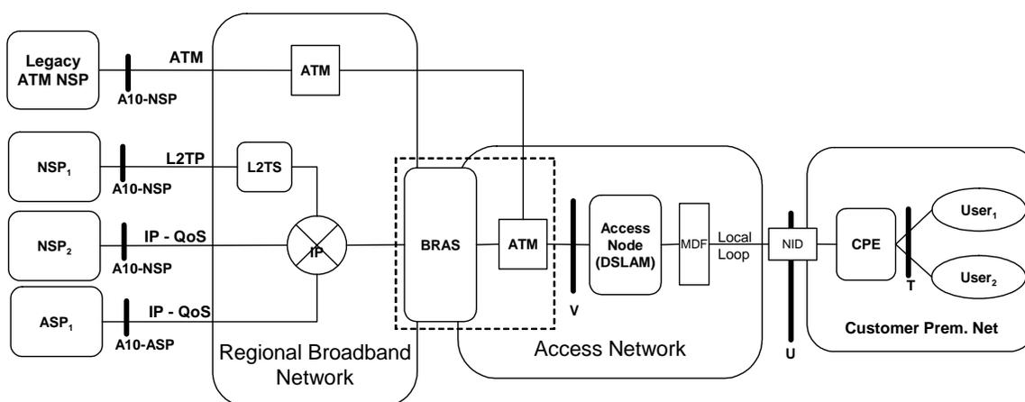
Figure 2- TR-059 High Level Architectural Reference Model
