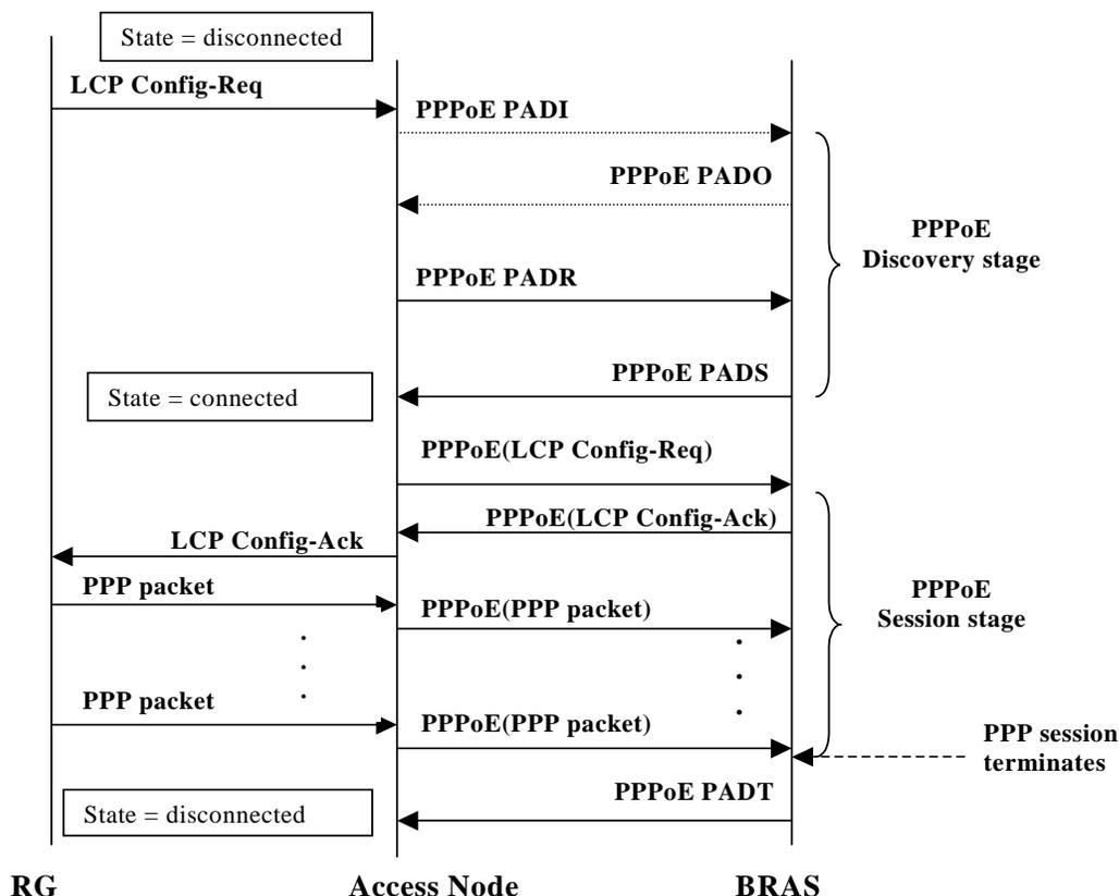
Figure 20 - Example message flow with PPPoA IWF
