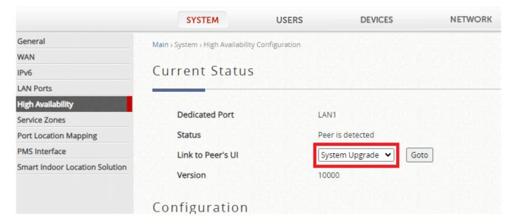
Step2: Upgrade firmware to Standby device again. (Standby HA sync will stop. It will show below message, doesn't need to RESTART Standby manually)
