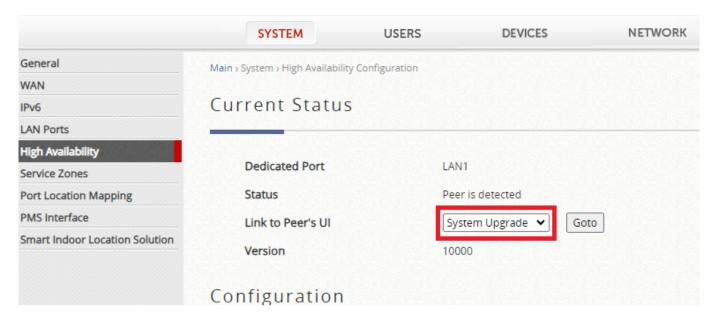
Step2: Upgrade firmware to Standby device again. (Standby HA sync will stop. It will show below message, doesn't need to RESTART standby manually)
