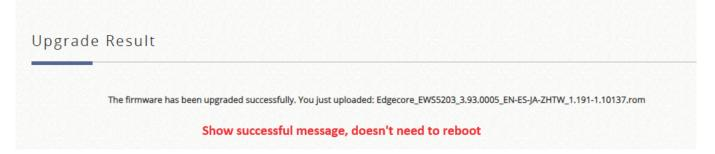
Step2: Upgrade firmware to Active and reboot Active (Standby will reboot automatically after 30 secs)
