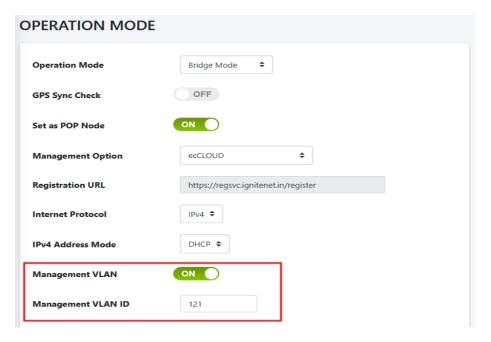
After configured on the POP node, the management VLAN settings will be automatically synchronized to other DNs and CNs connected under the POP node. All nodes in the same Terragraph network will be set with the same management VLAN ID.
