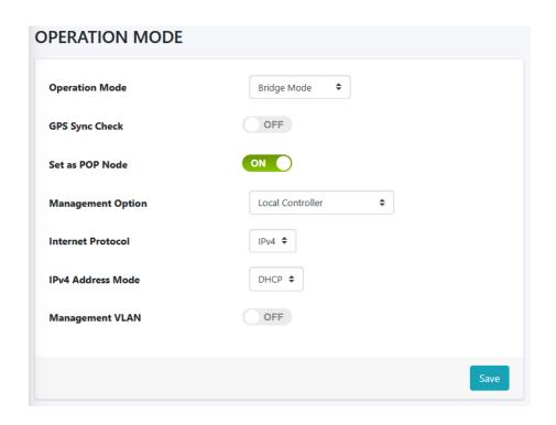
"Control Interface" is renamed as "Reserved Interface" now. The reserved interface is required when the Internet protocol is IPv6. The reserved interface is only for management purpose, and will be assigned with the control address. It can only be used to access the web GUI of the POP node.
