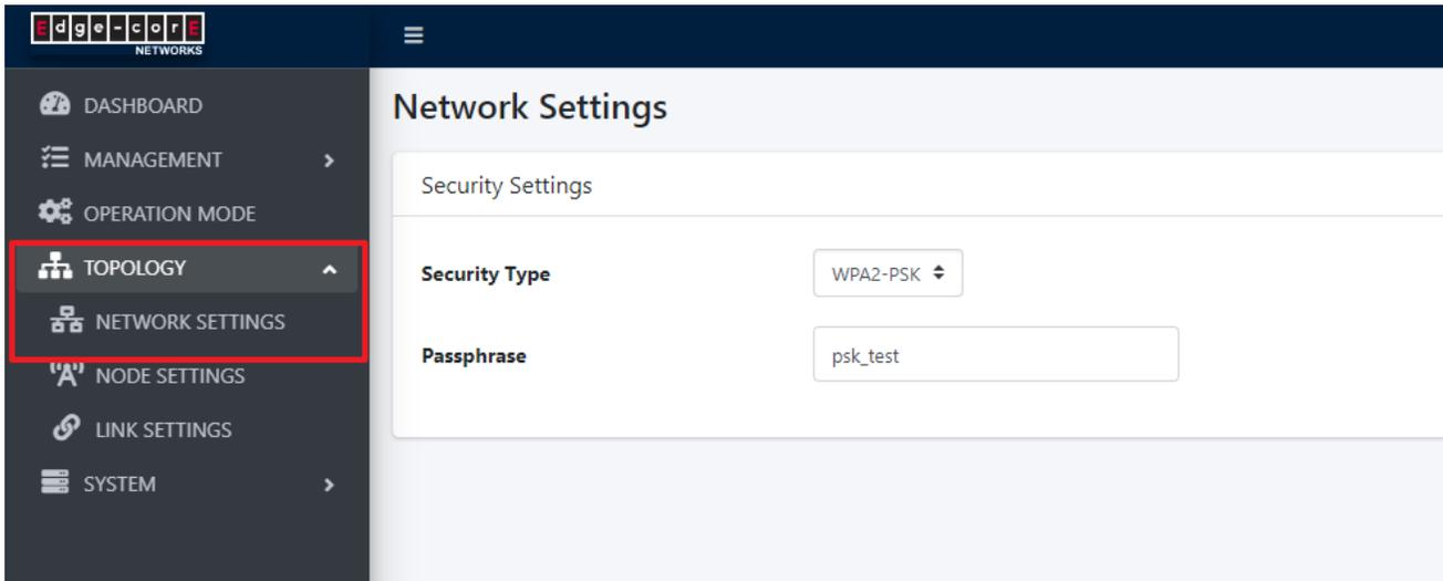
In current version, WPA2-PSK is the only supported security type. Passphrase is configurable and will be applied to all links of the node. The security settings must be the same for the two peers of a link. If the passphrase does not match, then the link cannot be established.
